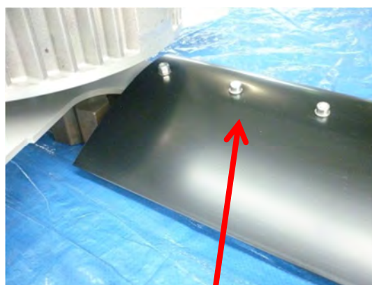
Blade's top face fixed with selflocking Bolts
